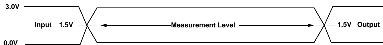
Figure 15. Input Waveforms and Measurement Levels
