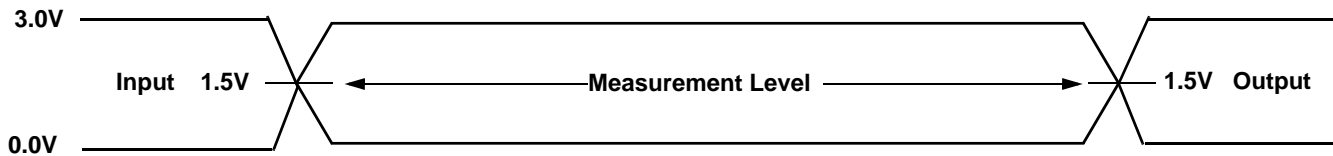
Figure 15. Input Waveforms and Measurement Levels
