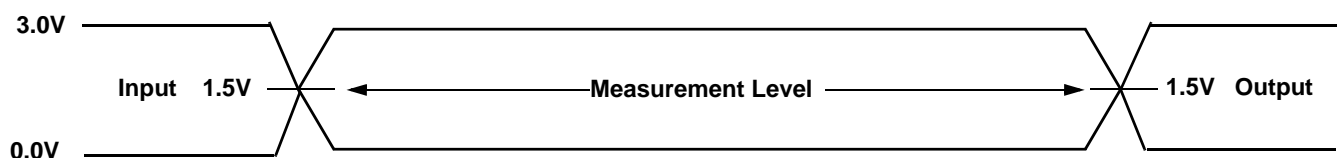
Figure 15. Input Waveforms and Measurement Levels
